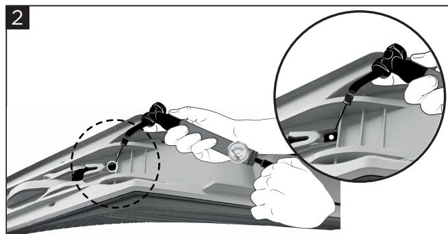
**To inflate the internal bladder connect the included needle tip to the pump and insert into the seat. For best results lube the needle with a silicone based lubricant.**
